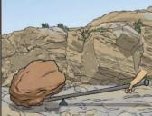
Levers can be used to make a small force lift a heavier load. A lever always rests on a pivot.
